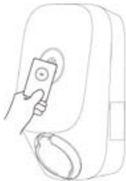
Figure 4-14 Charging by card swiping
